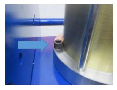
To remove the screw, loosen the hex nuts shown below. This will allow the screw to be removed.
