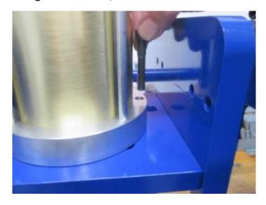
The cylinder can now safely be removed from the frame. Please not that this is a Model 400, but the same applies to all Direct Aire Models.
