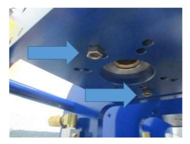
After loosening the hex nuts, remove the screws as shown below.
