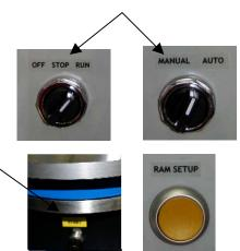
**Rotary Table Only** - Set Off-Stop-Run switch to STOP position and Manual-Auto switch to MANUAL. Set ROTARY TABLE ONLY toggle switch to the up position. Press the START button, the rotary table will index one position and stop, the ram will remain up. Press START to repeat.
